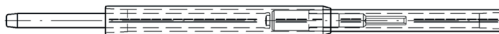
Compression joint for the connection of a hollow conductor with an Aluminium-Steel conductor
