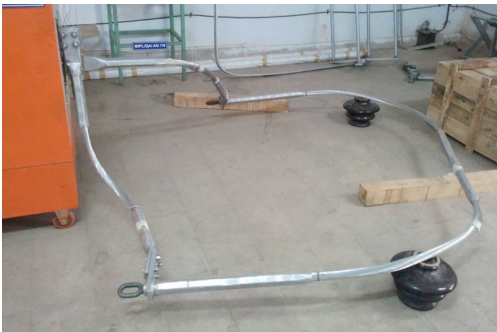
Ageing test with compression dead end clamps for high-temperature carrying conductors in the laboratory
